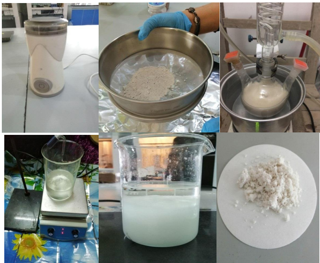
Figure (3.3):Shows steps of the preparation of \text{Al}_2\text{O}_3
